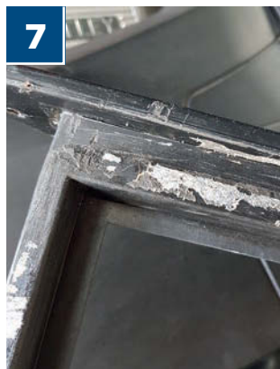
You must remove any old adhesive and dirt from each cartridge before refitting; Dan used carb cleaner to soften the glue and a sharp blade to clear it from the plastic surface
