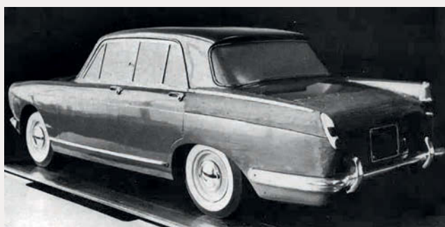
A quarter-scale Java model showing revisions to the rear bodywork, including the scaled-back fins
