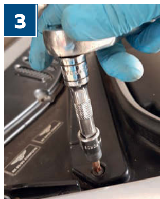
The pollen filters are positioned either side of the engine bay, close to the bulkhead – held in their own cartridges and accessed by undoing the two crosshead screws holding the cartridges in place
