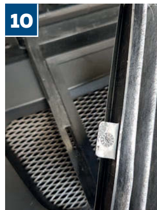
With the upper seal in place, insert a new pollen filter in each cartridge; genuine filters feature a tab to slot into a corresponding hole on the cartridge, which prevents incorrect fitting
