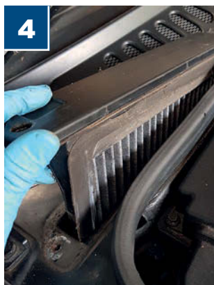
Take care when removing the cartridges, as they're a tight fit and not made of the world's sturdiest plastic; you'll need to reinsert them with the new filters and seals in place
