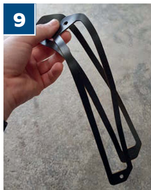
These are the genuine Bentley seals that need to be fixed to the underside of each filter cartridge's upper frame; take your time to align and press the parts into place, as they can tear and stick together easily
