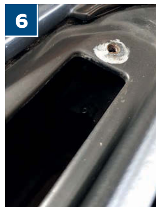
With the filters and cartridges removed, take time to clean the cartridge mating surface in the engine bay; it makes sense to do this now, as access is obviously that much easier
